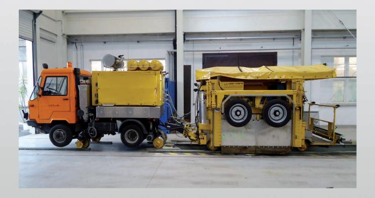
The RRGM 1-6/ AM 65 is a road-rail going grinding machine for the machining of the rail head of tracks and turnouts. It composes except the grinding wagon also a generator so that no power cables has to be installed along the working site. The grinder can travel flexibly to the position for rail-in und easily rail in and out by road-rail technology.
