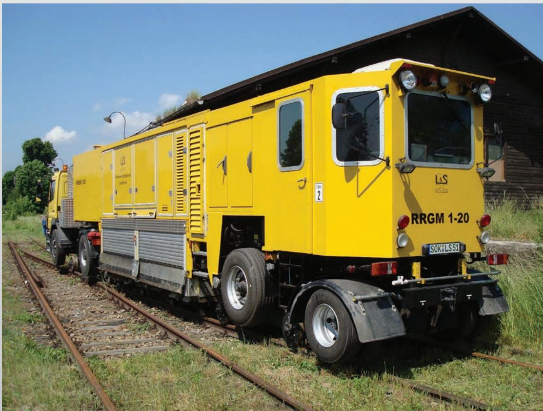
The rail grinder RRGM 1-20 is a rail-road going machine. The machine has 20 grinding motors with independent angular adjustment. They are driven by 7,5 to 15 kW frequency-controlled electrical motors. The computer monitored grinding process is controlled with touch pad by the operator inside of the cabin.
