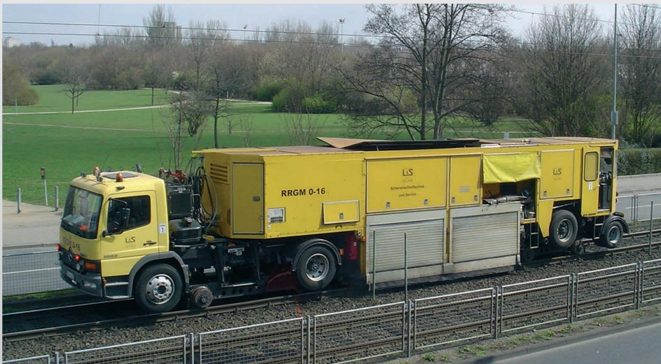
The rail grinder RRGM 0-16 is a rail-road going machine. The machine has 16 grinding motors with independent angular adjustment. They are driven by frequency-controlled electrical 7,5 kW motors. The computer monitored grinding process is controlled with touch pad by the operator inside of the cabin.
