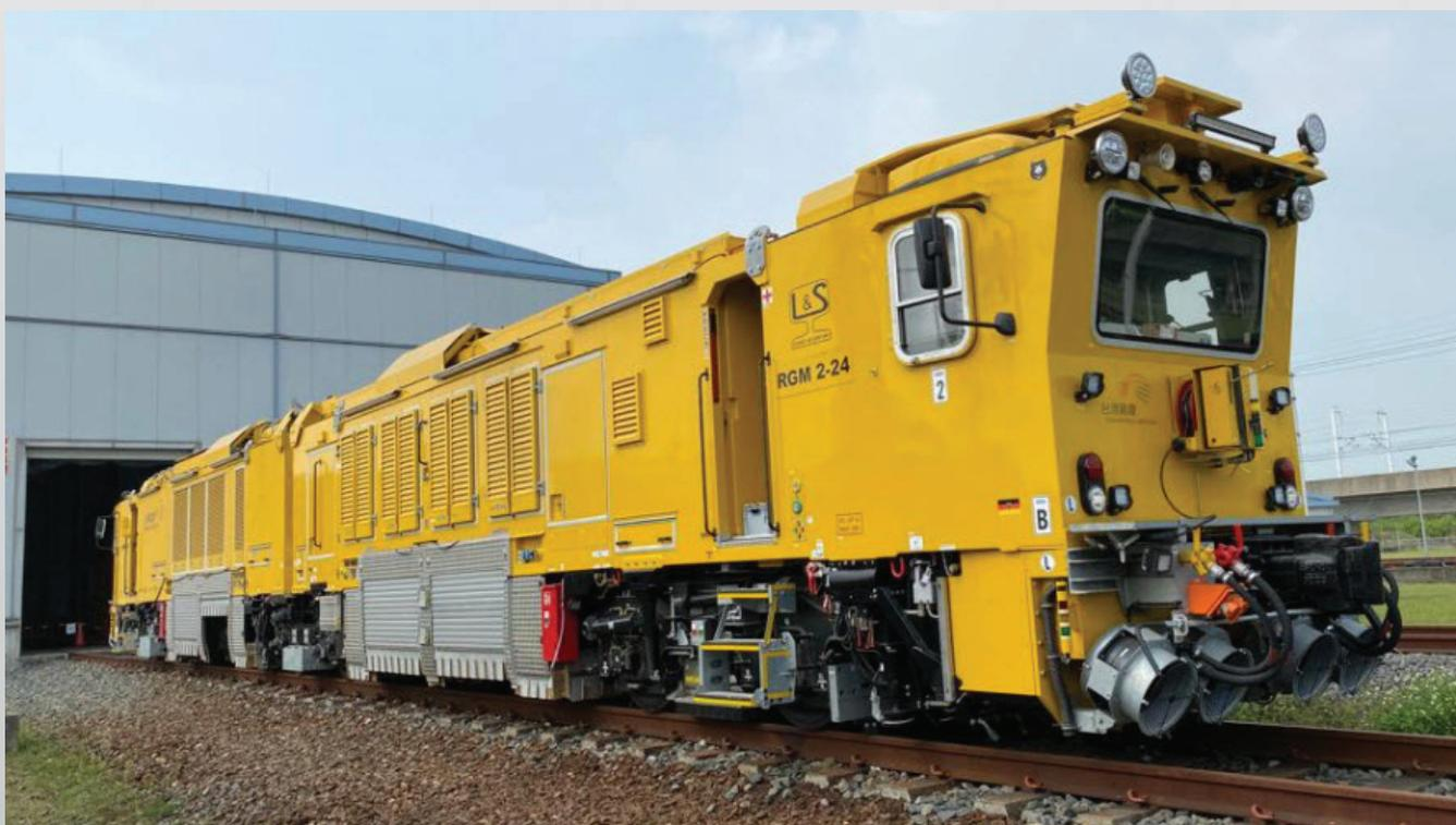
The rail grinder RGM 2-24 is a rail-borne machine which is consisted of two wagons and has 24 grinding motors with independant angular adjustment. Each of the spindles is driven by a frequency-controlled electrical motor. The computer monitored grinding process is controlled with touch pad by the operator inside of the cabin.
