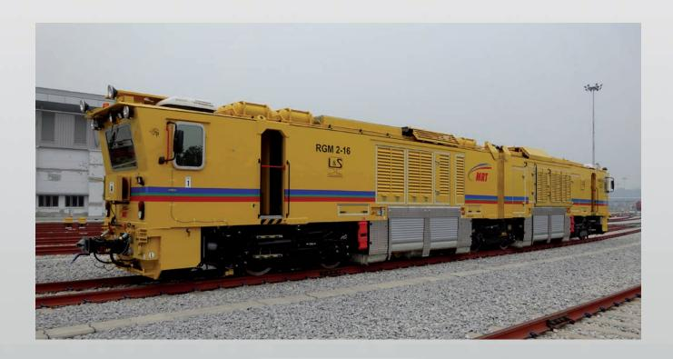
The rail grinder RGM 2-16 is a rail-borne machine which is consisted of two wagons and has 16 grinding motors with independant angular adjustment. Each of the spindles is driven by a frequency-controlled electrical motor. The computer monitored grinding process is controlled with touch pad by the operator inside of the cabin.
