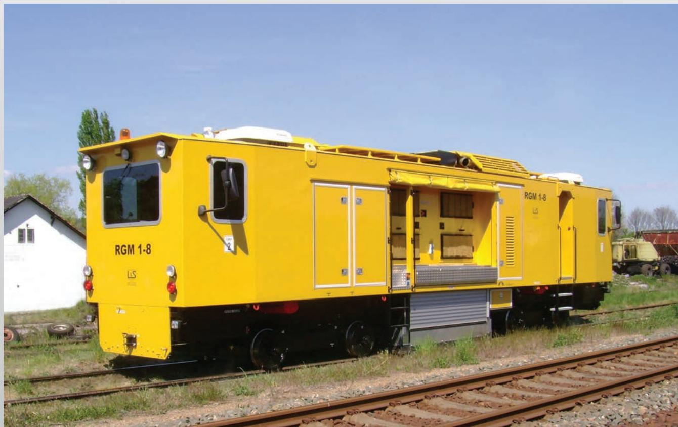
The rail grinder RGM 1-8 is a rail-borne machine which has 8 grinding motors with independant angular adjustment. Each of the spindles is driven by a frequency-controlled electrical motor. The computer monitored grinding process is controlled with touch pad by the operator inside of the cabin.
