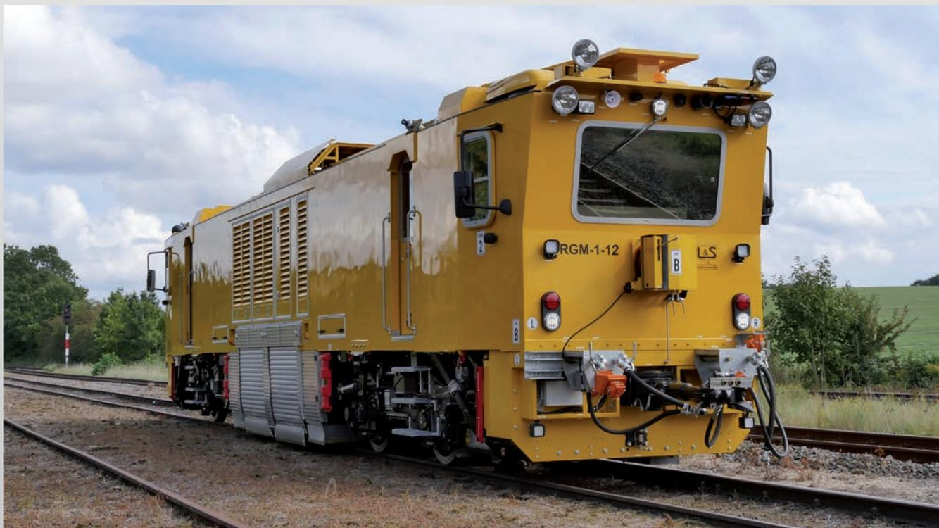
The rail grinder RGM 1-12 is a rail-borne machine which has 12 grinding motors with independent angular adjustment. Each of the spindles is driven by a frequency-controlled electrical motor. The computer monitored grinding process is controlled with touch pad by the operator inside of the cabin.
