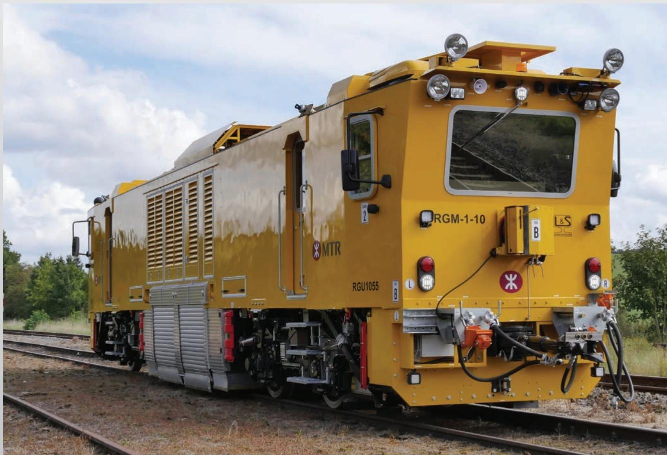
The rail grinder RGM 1-10 is a rail-borne machine which has 10 grinding motors with independant angular adjustment. Each of the spindles is driven by a frequency-controlled electrical motor. The computer monitored grinding process is controlled with touch pad by the operator inside of the cabin.
