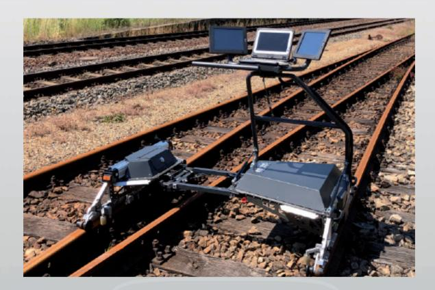
The LTMD 2-4-HC is an efficient solution for continuous measurement on tracks as well as for continuous or point measurement in switches. The online measuring device LTMD 2-4-HC can be used for grooved rails and standard Vignol rails in track systems with track gauges 900-1435 mm and enables simultaneous measurement of the left and right rails. The following measuring methods are integrated:
