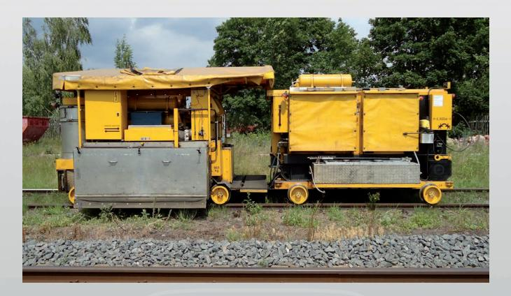
The LRGM 1-6/ AM65 is a plain track and a turnout grinding machine for the machining of the rail head which composes except the grinding unit also a generator so that no power cables has to be installed along the working site. The grinder can be easily railed in and out with a ramp of a rail vehicle or by crane.
