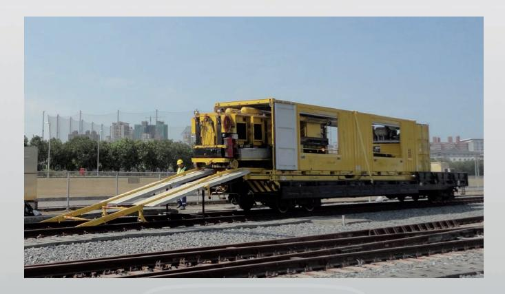
The CRIO System is a container transport and loading system for movable machines providing control and maintenance works in railway track systems. The system enables a very flexible and direct transport to the working site, a fast transfer to and from rail tracks and an easy switchover to the next maintenance site.
