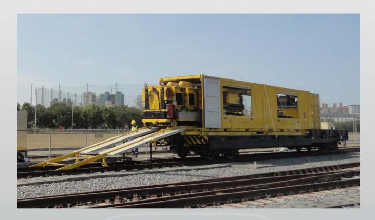
The CRIO Container System is a transport and loading system for movable machines providing control and maintenance works in railway track systems. The system enables a very flexible and direct transport to the working site, a fast transfer to and from rail tracks and an easy switchover to the next maintenance site.
