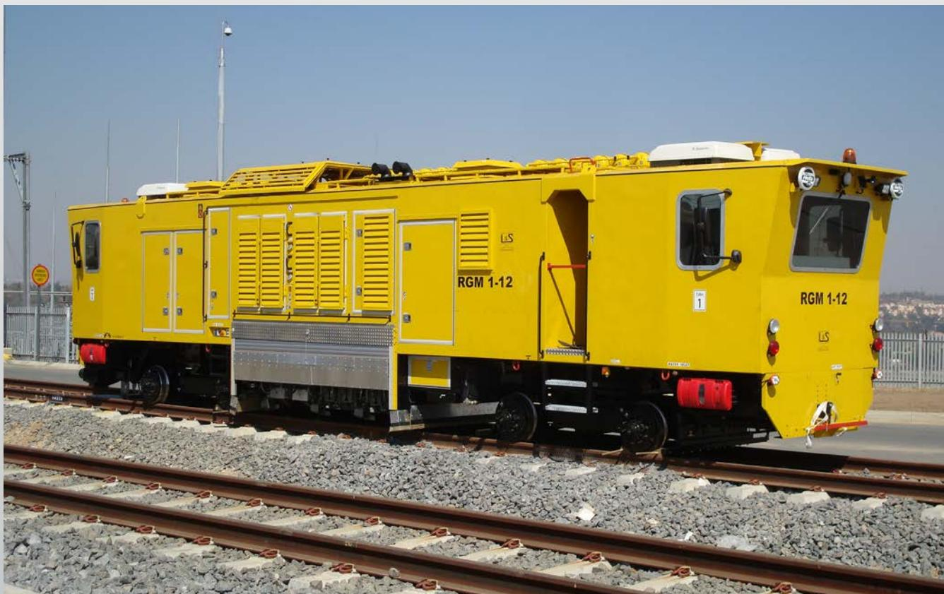
The rail grinder RGM 1-12 is a rail-borne machine which has 12 grinding spindles with independent angular adjustment. Each of the spindles is driven by a frequency-controlled electrical motor. The computer monitored grinding process is controlled with touch pad by the operator inside of the cabin.
