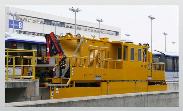
The Maintenance Inspection Vehicle MIV 1-25 is designed for use on monorail system for track inspection and maintenance work. The Maintenance Inspection Vehicle is applicated for
